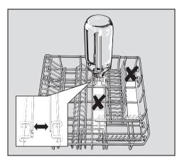
The bottle holder can be placed in any area marked in white in the illustration below. Do not place it in the areas marked with an X, these areas will not receive adequate water coverage.
